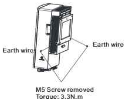
Figure 3.7 Connect the external grounding conductor
